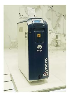
The big difference compared to the traditional method consists of the fact that the Syncro control unit supplies cold water to the mold **only** during the cooling phase, drastically reducing its duration. The advantages for the customer are easily understood: increased productivity and profitability of the dedicated production cell, against an investment with an average payback time of less than 6 months.
