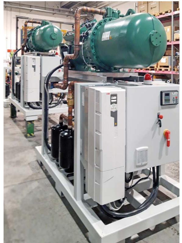
To achieve very accurate control of compressors and pumps, and consequently accurate adjustment of the cooling capacity, Frigel has adopted ABB's ACS580 drive, combined with ACS310 auxiliary units mounted on the pumping groups to circulate the coolant fluid between chiller and users. Each drive is controlled by a PLC programmed with proprietary logic.
